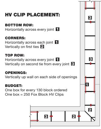
Using the Fox Blocks HV clip eliminates the need for truss wire completely on your jobs. The result is that for about 1/2 the cost of the truss wire you will get a stronger and straighter job.
